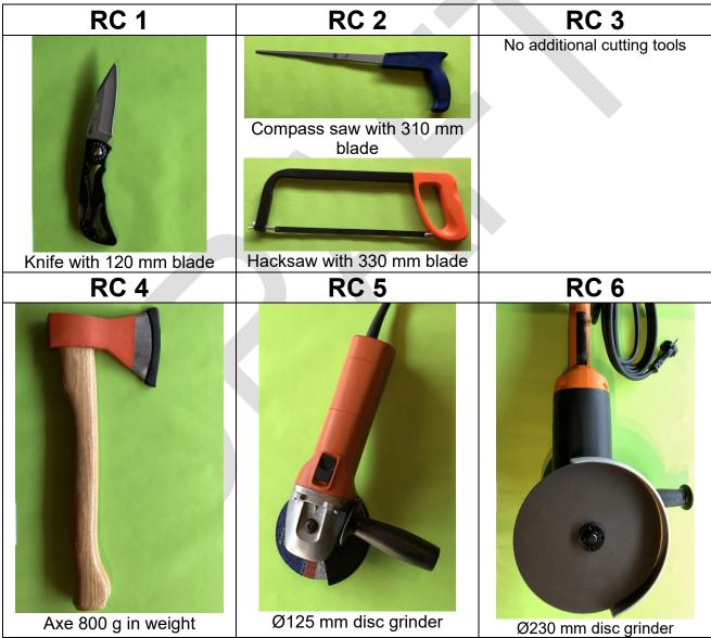
Burglary tools used in EN 1630 to cut the products per class (the tools of RC 1 can also be used in RC 2, RC 3 etc, the tools of RC 2 can also be used in RC 3, RC 4 etc.)
